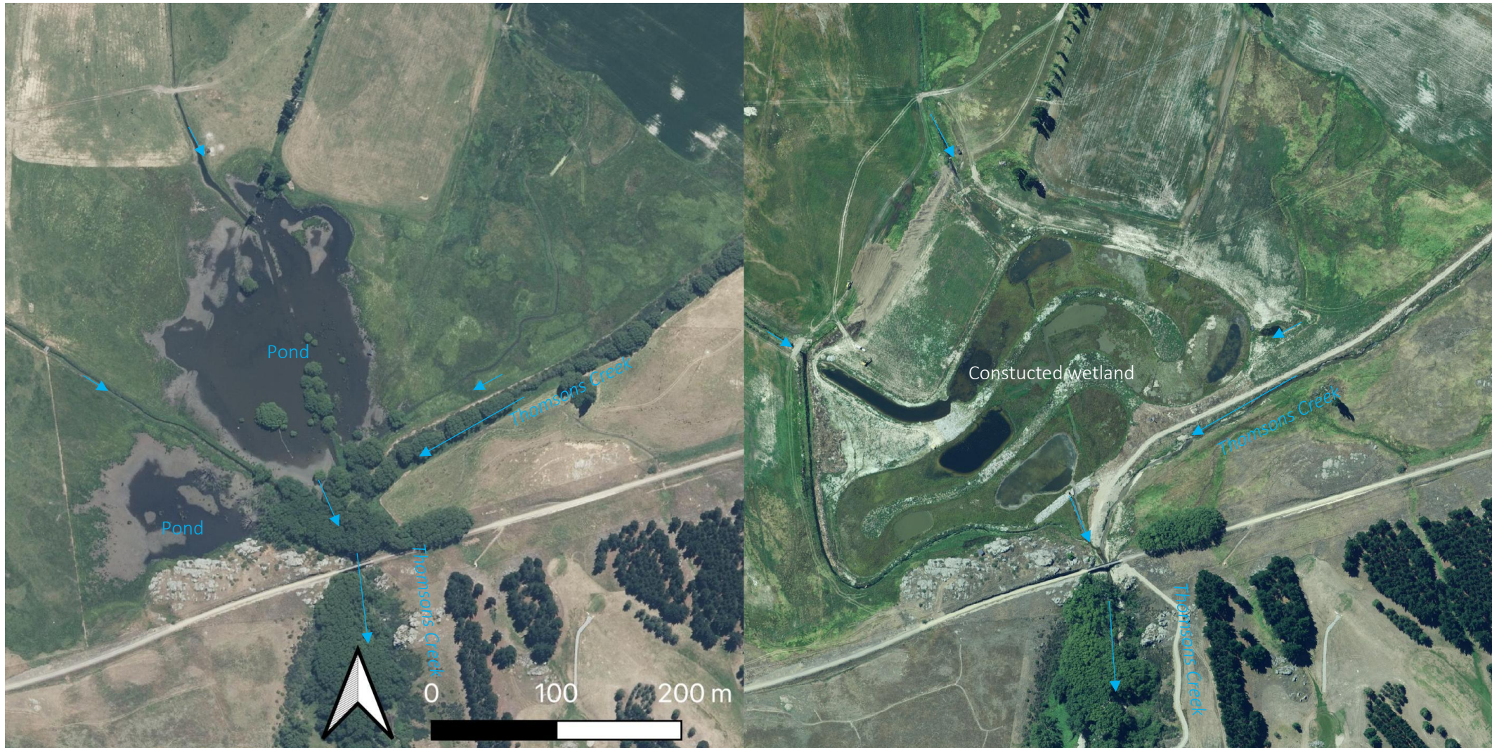
Figure 2 Aerial photographs of the lower Sluice Channel prior to (left) and immediately after (right) the construction of the constructed wetland.
